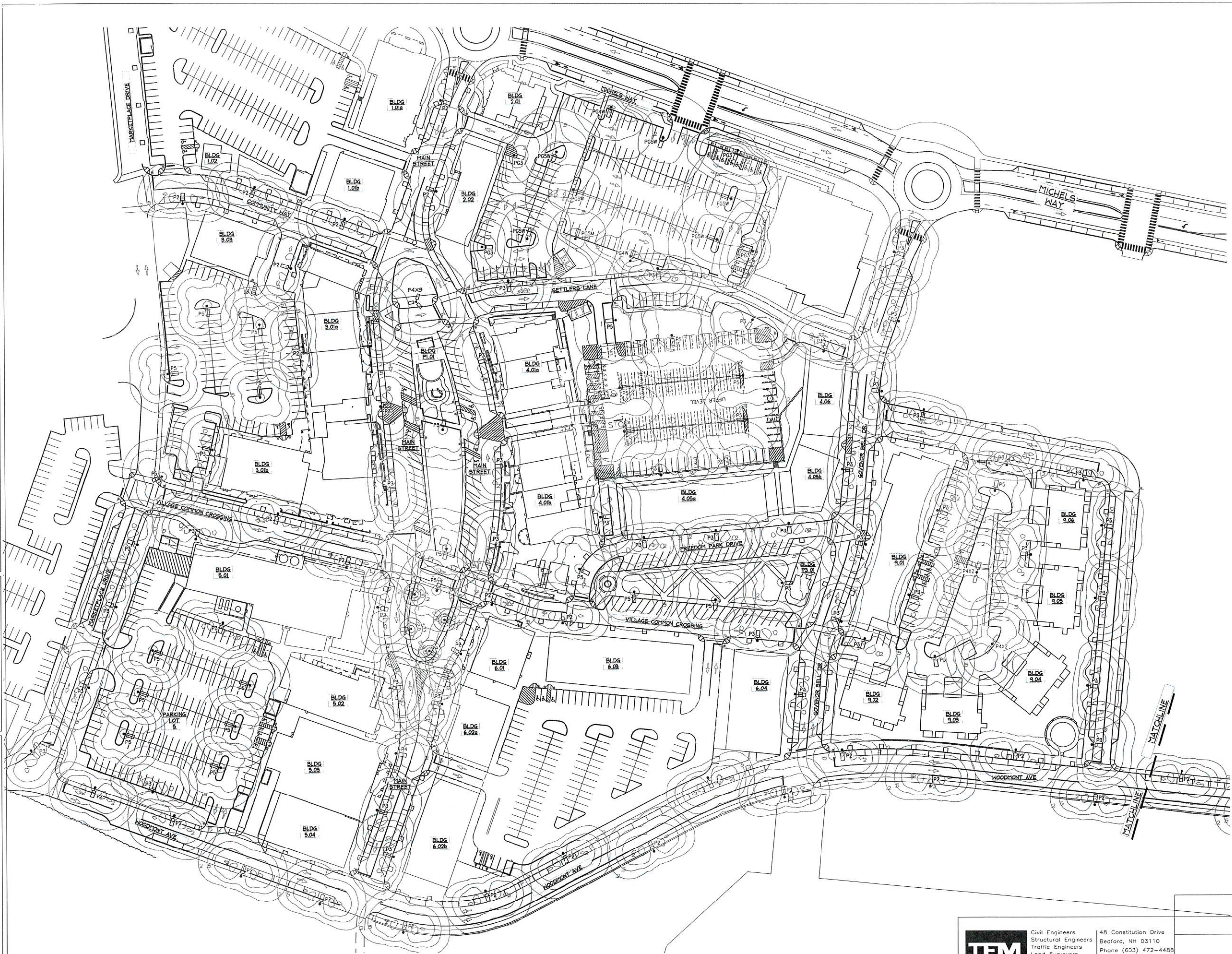
PHASE 1 SITE PLAN - ISO FOOTCANDLE DISPLAY SCALE: 1" = 60'-0"
